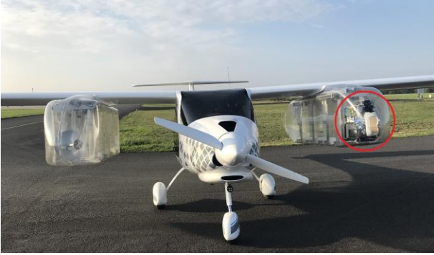
Figure 7: The test aircraft, with the radar in the front of the port freight container
