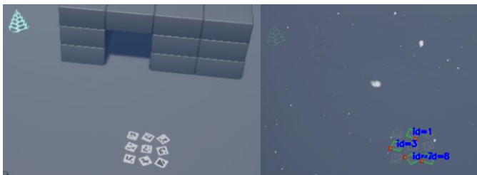
Figure 4 left: no weather; right: snow, dust and fog combined, 4 out of 9 markers detected
