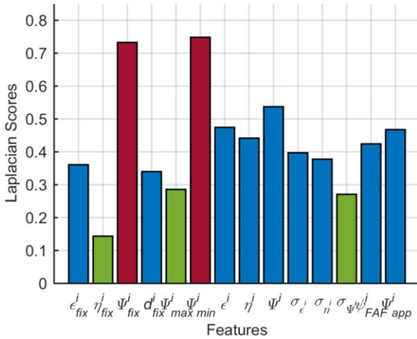
Figure 5. Illustration of Laplacian Scores
