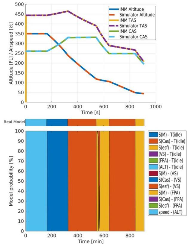
Figure 1. Simulated and IMM estimated aircraft descent trajectory (top), real guidance mode (middle) and IMM mode probability (bottom).
