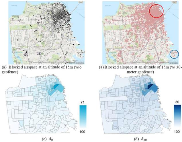
Fig. 2 Several maps of airspace availability in San Francisco. (a): Blocked airspace at an altitude of 15-meter without geofence, (b): Blocked airspace at an altitude of 15m with 30-meter geofence, (c):Thematic map of  $A_0$ , (d): Thematic map of  $A_{30}$
