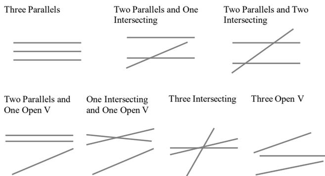
Figure 4 Seven Types of Three Runway Configurations
