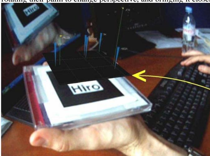
Figure 1. AR in your hand. A section of the airspace is depicted in 3D. The image is anchored to the marker, so moving the marker moves the 3D information as well. This allows views from multiple directions and collaboration between controllers.
