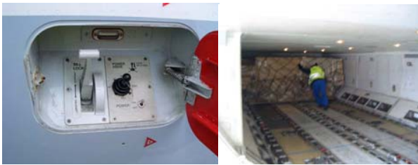
Figure 5. Physical Deficiencies : Displaced Control Panel for cargo door (left) / Manual positioning of load compartment (right)
