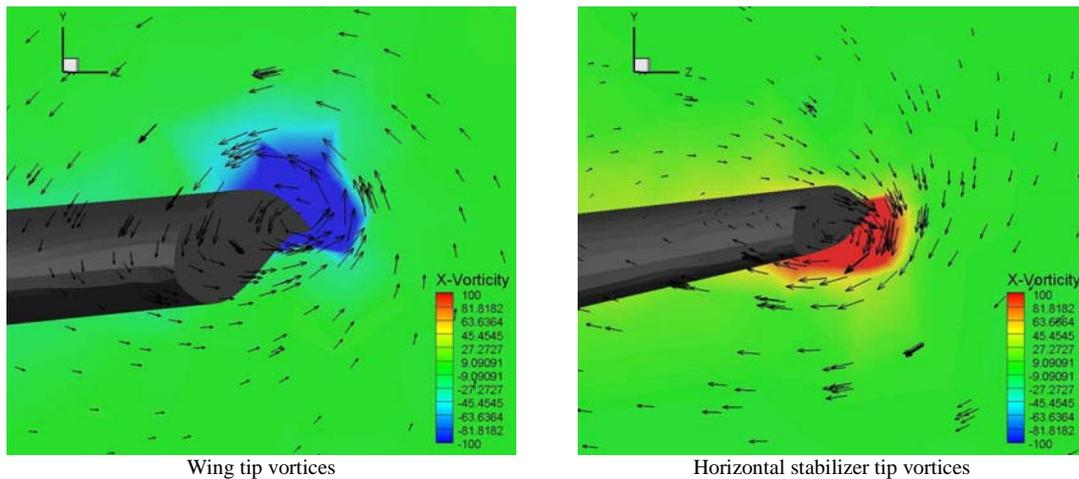
Figure 7. Wing and horizontal stabilizer tip vortices comparison
