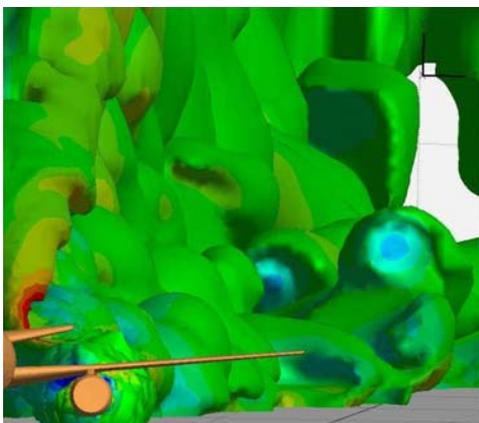
Figure 8. Iso-surface of 1ppm of NO<sub>x</sub> plotted with x-vorticity
