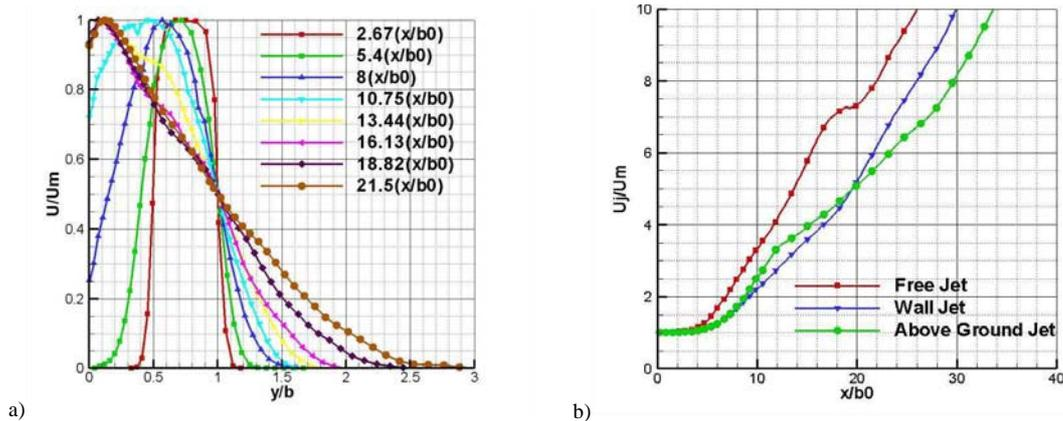
Figure 5. Vertical velocity profile (a) and velocity decay comparison between different jets (b)
