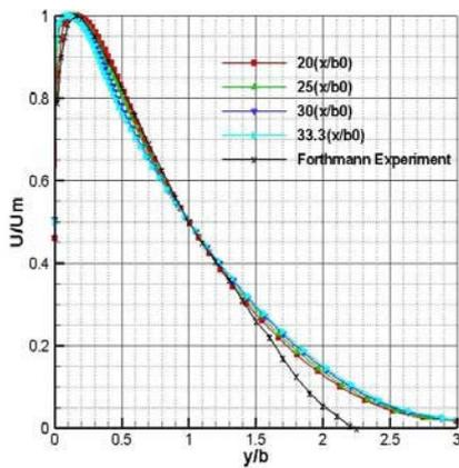
Figure 3. CFD and experimental results for the non buoyant wall jet vertical velocity profile
