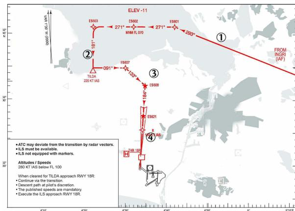
Fig. 1. The approach route, top view. The starting points of the phases of the CDA procedure are indicated. ① Level flight at FL70, ② Constant IAS descent along  $3^\circ$  glide path, ③ Idle thrust descent, ④ Constant final approach speed along ILS.
