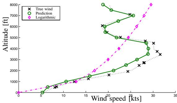
Fig. 4. Wind profile prediction performance. A typical wind profile and its estimate (in 500 ft intervals). For reference, a best-fit logarithmic profile is also shown.
