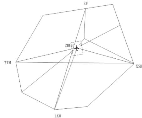
Figure 1. Airspace structure in Wuhan approach. The main fixes are ZF, WTM, LKO, and XSH. Departure/arrival traffic from/to Wuhan airport are all through these fixes.
