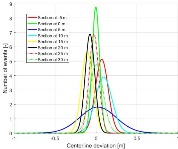
Figure 12 The Gaussian functions at various cross sections fitted to the centerline deviation histogram
