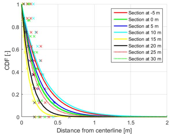
Figure 13. Relative histogram of the aircraft-centerline distances at different cross sections.
