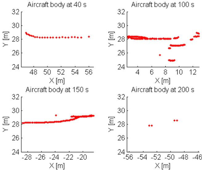
Figure 4. Backscattered points from the aircraft body at various times from the same sensor
