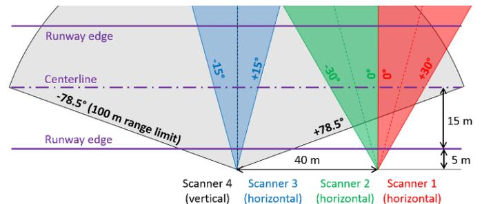
Figure 2. Four scanner configuration (drawing not to scale)
