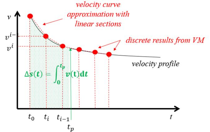
Figure 5. Approximation of the velocity curve with discrete samples obtained by constant model (CV)
