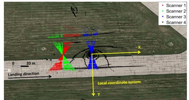
Figure 8. Acquired point clouds (top view)
