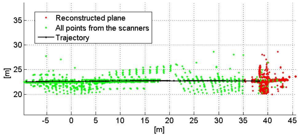
Figure 9. Reconstructed plane cloud, including all points from the sensors and the estimated trajectory
