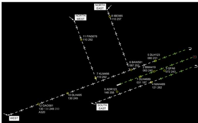
Figure 4. Rectangular display route structure for better comparison of aircraft on different routes (Display 5).
