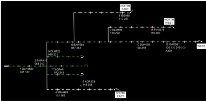
Figure 7. Unidirectional orthogonal monitoring display with the runway on the left side and downwind flights to be avoided (Display 9).
