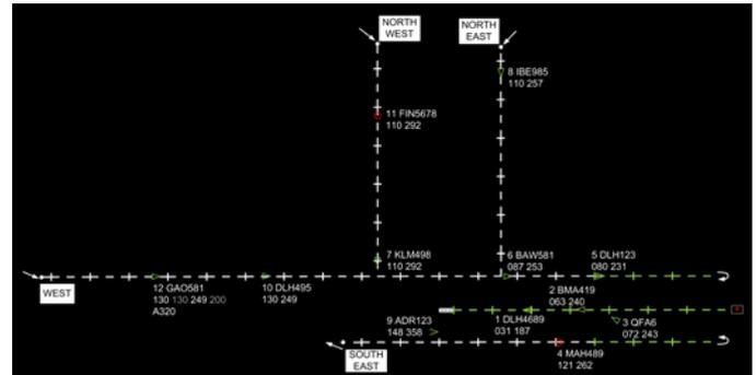
Figure 5. Orthogonal displayed route structure with aircraft symbology for optimization purposes (Display 7).
