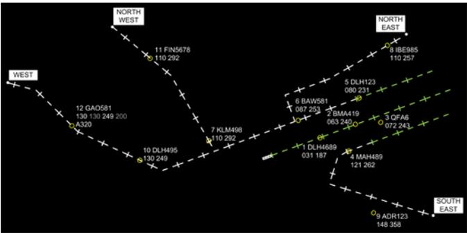
Figure 2. Distance marking at STARs on a currently usable controller display with a runway in the middle and four initial approach fixes (Display 1).
