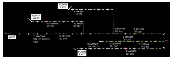
Figure 6. Parallelized displayed route structure with straightened merge points for comparison of all incoming routes (Display 8).
