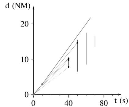
Figure 5. Exploration of the decision tree. For each time step, 3 choices are tested: to accelerate, to cruise, to decelerate. The choice leading to the longest conflict-free trajectory is applied (in this case, it accelerates two times at the beginning, then it cruises).
