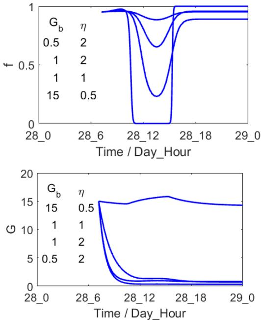
Figure 6. Simulation of performance disruption  $f(t)$  (top) and recovery action  $G(t)$  (bottom) dependent on offset  $G_b$  and time constant ratio  $\eta$ . Disturbance  $w(t)$  from “Christian”. Model parameters  $v_{th} = 18$ ,  $[dv/dt]_0 = 35$ ,  $\tau_0 = \tau_r = 1.5$  h,  $f_0 = 0.95$ ,  $f_b = 0.6$ ,  $\eta = 0.5$ ,  $G_0 = 15$ . Succession of curves corresponds to that of  $[G_b, \eta]$ -parameter values
