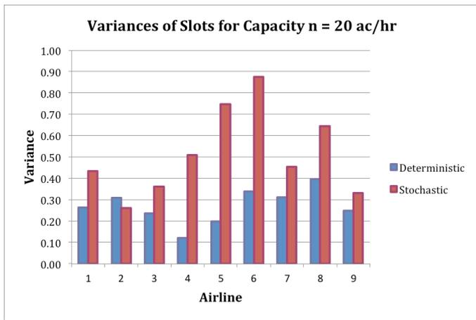
Figure 8. Variance of slots when capacity is reduced to 20 ac/hr
