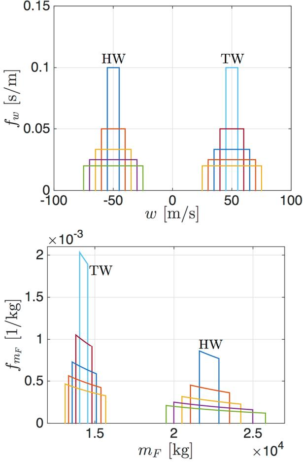
Figure 5. Fuel mass pdf for different wind distributions: HW  $\bar{w} = -50$  m/s and TW  $\bar{w} = 50$  m/s;  $\delta_w = 10, 15, 20, 25$  m/s.
