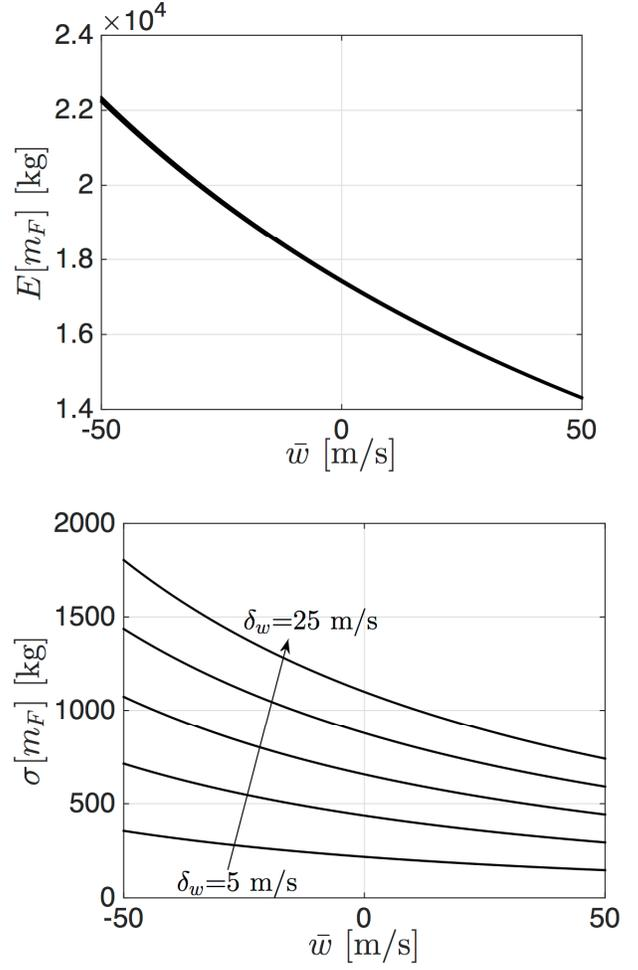
Figure 6.  $E[m_F]$  and  $\sigma[m_F]$  as a function of  $\bar{w}$ ;  $\delta_w = 5, 10, 15, 20, 25$  m/s.
