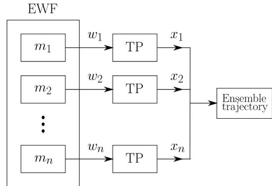
Figure 1. Ensemble trajectory prediction. Legend:  $m$  - member,  $w$  - weather,  $x$  - trajectory.
