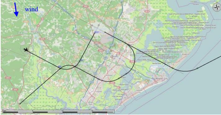
Figure 1. Different approach trajectories with RTAs for each waypoint.
