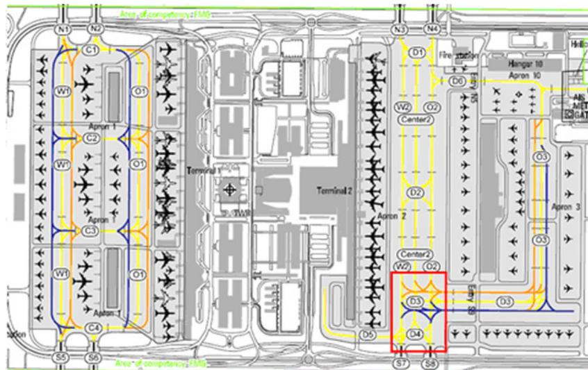
Figure 1. Apron layout at Munich Airport [1]
