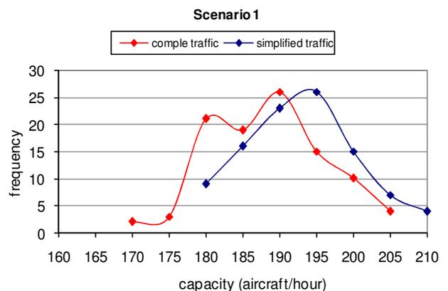
Figure 9. Simulation results with complete and simplified traffic data, Scenario 1
