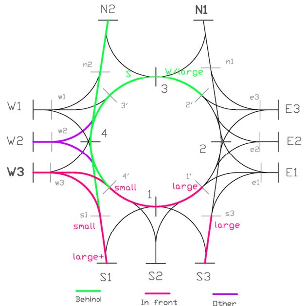
Figure 6. Restricted sections for West-North-small aircraft
