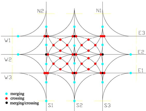
Figure 5. Merging and crossing points in the conventional intersection
