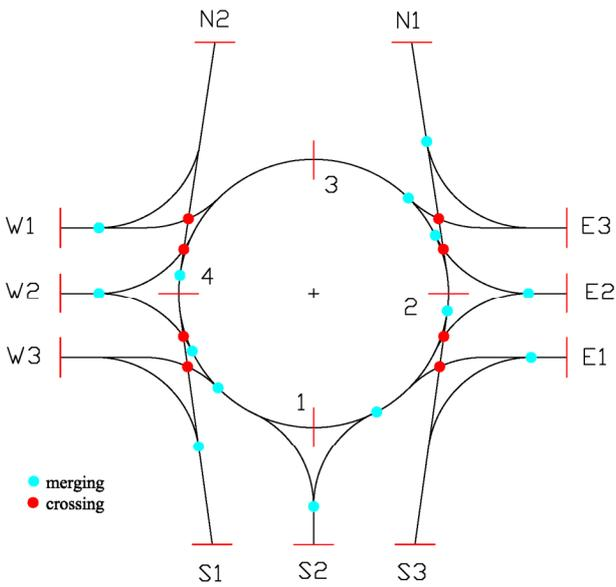
Figure 4. Merging and crossing points in the roundabout
