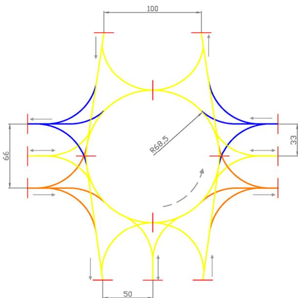
Figure 2. The roundabout geometry – preliminary design
