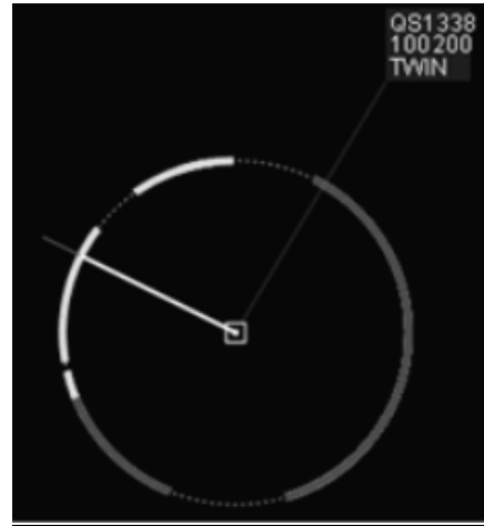
Figure 1. Close-up of the SSD screen showing GO, NO-GO short term conflict and NO-GO medium term conflict headings.
