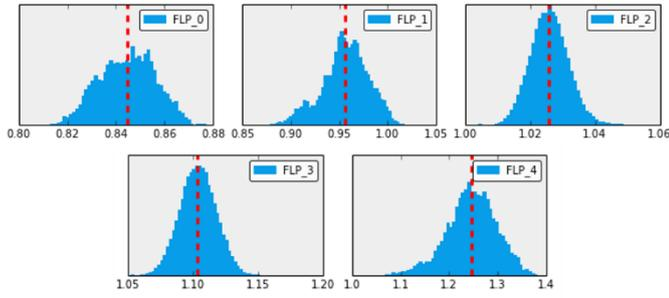
Figure 6. Lift coefficient distribution due to flap deflection
