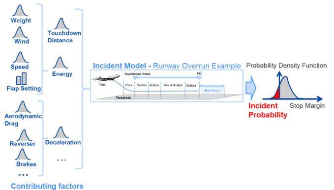
Figure 4. Propagation of probability distributions through a physical model
