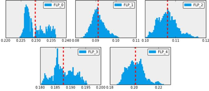
Figure 7. Drag coefficient distribution due to flap deflection
