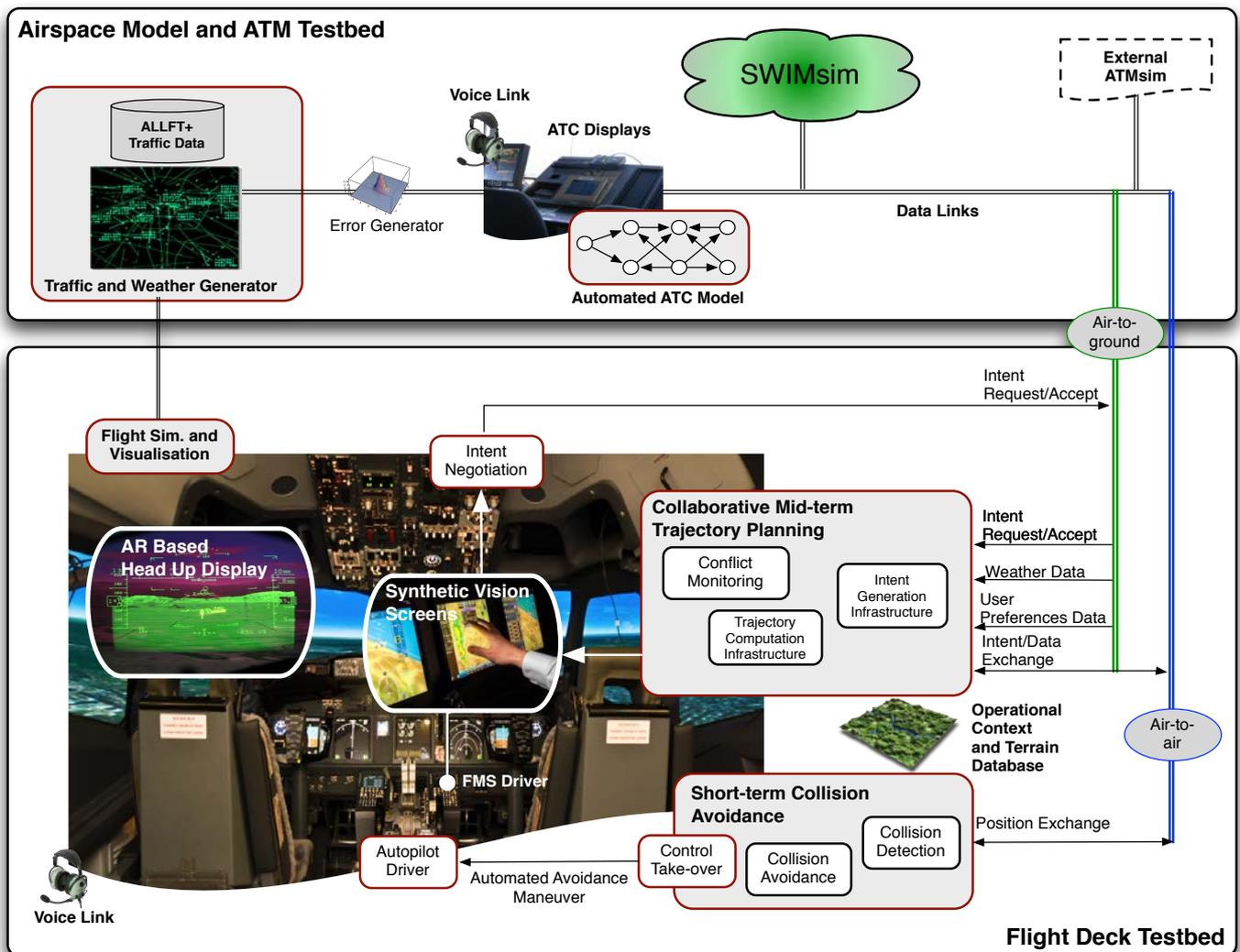
Figure 3. Architecture of the integrated next generation flight deck system with novel add-on modules
