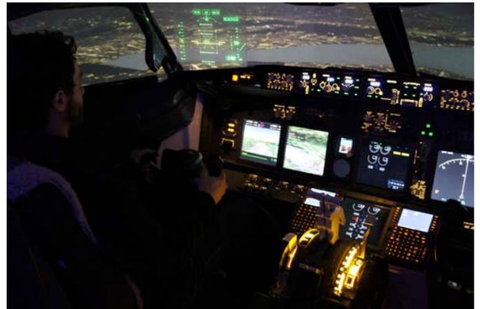
Figure 1. B737-800 flight deck platform with experimental visual decision support tools
