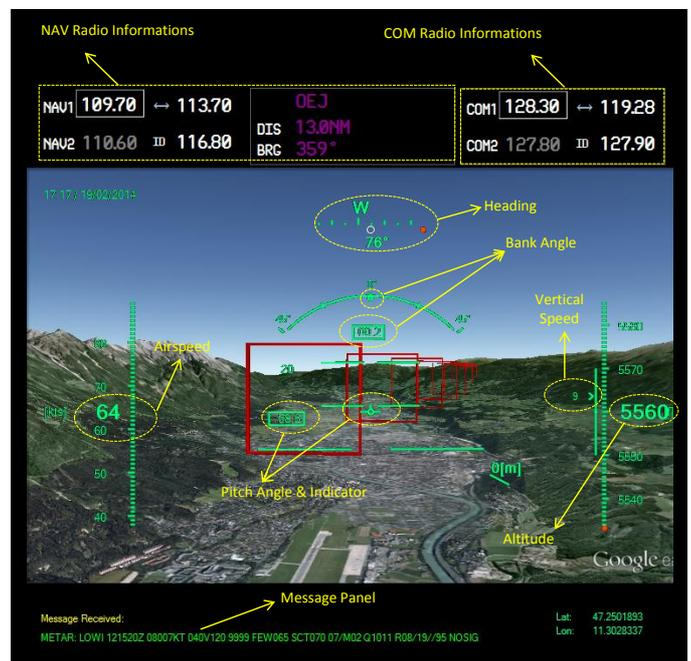
Figure 7. Definitions of the symbology in Synthetic Vision Display (SVD)
