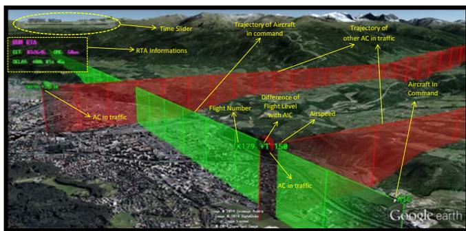
Figure 6. Definitions of the symbology in 4D Operational Display (4DOD)
