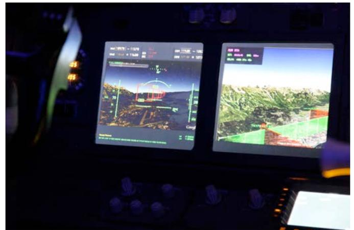
Figure 5. Synthetic Vision Display (SVD) and 4D Operational Display (4DOD) screens in the flight deck
