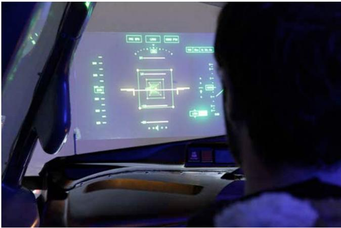
Figure 8. Transparent Screen overlay for HUD augmented reality implementations
