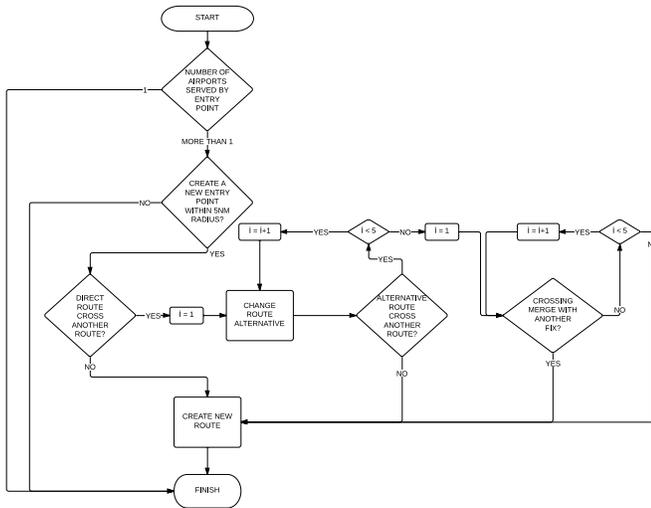
Fig. 1. Entry-point Multiplication Algorithm
