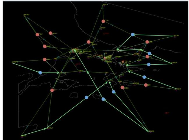
Fig. 2. Air space view with new entry points and routes.
