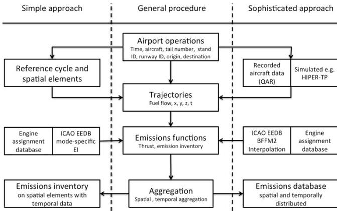
FIGURE II – GENERAL, SIMPLE AND SOPHISTICATED PROCEDURES FOR THE PREDICTION OF LTO ENVIRONMENTAL IMPACT
