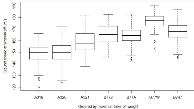
FIGURE IV – AIRCRAFT TYPE SEPARATED BOXPLOTS FOR GROUND SPEEDS AT WHEELS OFF
