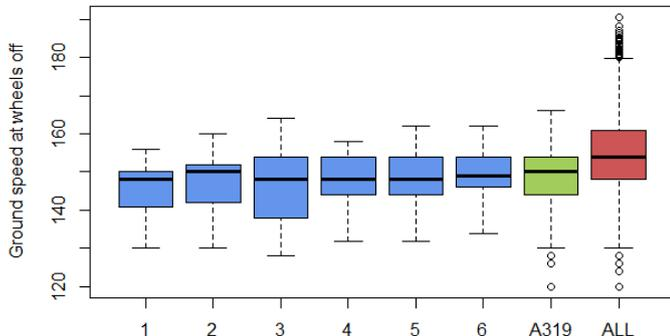
FIGURE VII - VARIATION IN GROUND SPEED AT WHEELS OFF OF SAME AIRCRAFT
