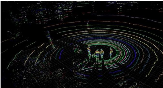
Figure 2. Visualization of point clouds applied to a segmentation filter with colour-coding
