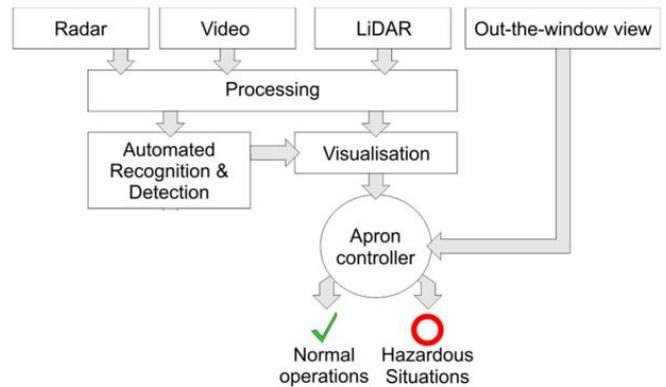
Figure 4. Sketch of the LiDAR-based surveillance concept
