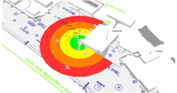
Figure 5. Theoretical coverage of OPAL 360 series at maximum PRR for an exemplary installation on the terminal roof of Dresden airport [Neptec Technologies, Canada; AIP DFS Deutsche Flugsicherung, Germany]
