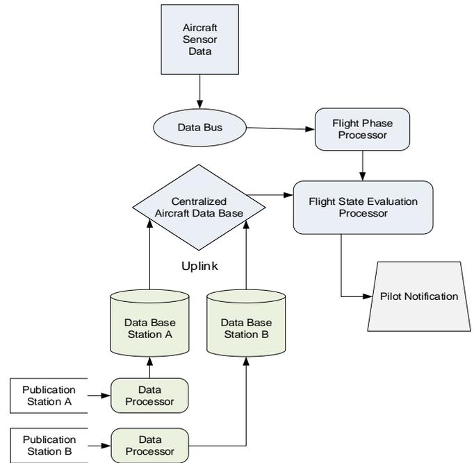
Figure 2. Flight State Evaluation, Data Processing
