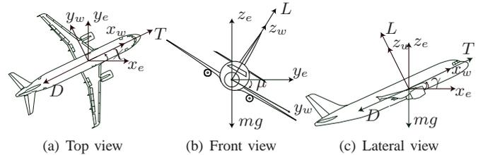
Fig. 1. Aircraft state and forces
