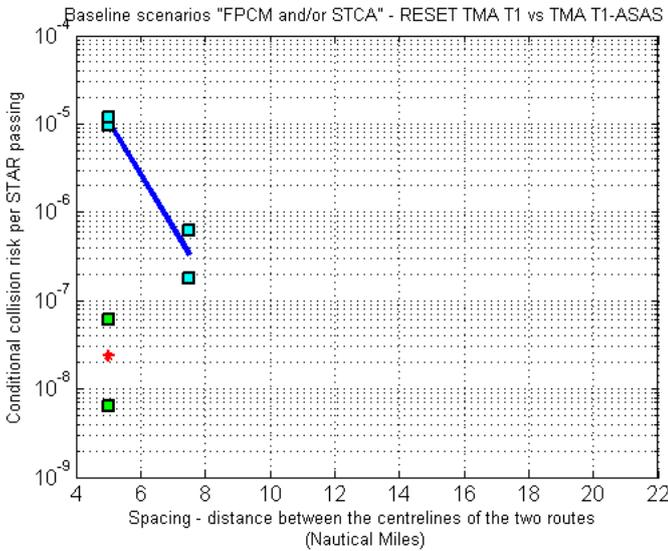
Figure 6. Monte Carlo simulation results for non-nominal encounter condition “FPCM and/or STCA” for TMA-T1 (upper, blue line) and TMA-T1-ASAS (lower, red dot). The small blue and green blocks indicate the upper bound and the lower bound of a 95% confidence interval.
