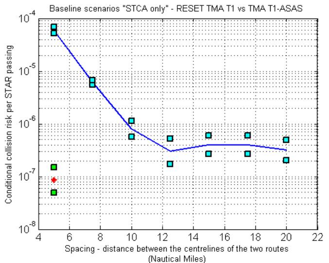
Figure 5. Monte Carlo simulation results for non-nominal encounter condition “STCA only” for TMA-T1 (upper, blue line) and TMA-T1-ASAS (lower, red dot). The small blue and green blocks indicate the upper bound and the lower bound of a 95% confidence interval.
