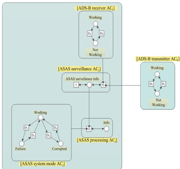
Figure 3. The agent in the TMA-T1-ASAS operation is modelled by five LPNs and a number of ordinary and enabling arcs. In this figure  $ac_j$  represents an aircraft on level ( $j=0$ ) or an aircraft on a STAR ( $j=1, \dots, m$ ), and  $k \neq j$ .
