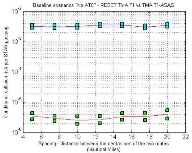
Figure 4. Monte Carlo simulation results for non-nominal encounter condition “No ATC” for TMA-T1 (upper, blue line) and TMA-T1-ASAS (lower, red line). The small blue and green blocks indicate the upper bound and the lower bound of a 95% confidence interval.
