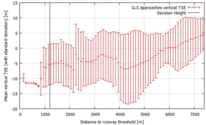
Figure 8: Mean vertical TSE during GLS approaches
