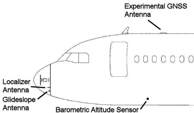
Figure 3: Approximate antenna and sensor positions
