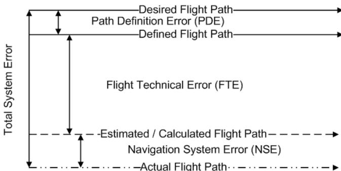
Figure 1: Flight Path Error Types
