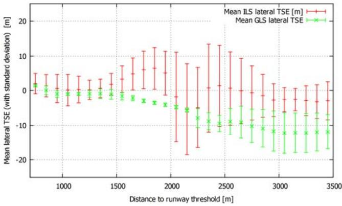
Figure 14: Comparison of mean lateral TSE during ILS (red) and GLS (green) approaches
