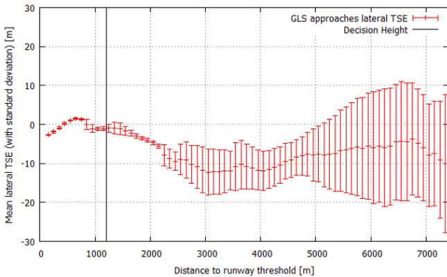
Figure 7: Mean lateral TSE during GLS approaches
