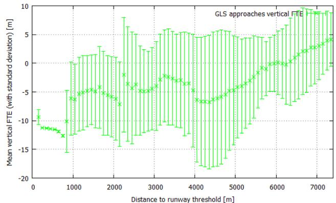
Figure 10: Mean vertical FTE during GLS approaches
