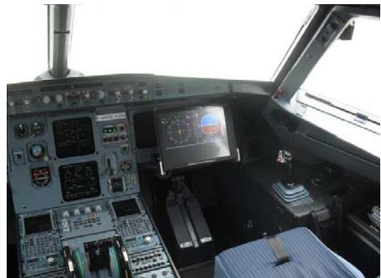
Figure 2: ATRA experimental cockpit display
