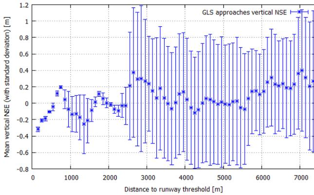
Figure 12: Mean vertical NSE during GLS approaches
