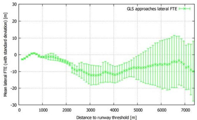
Figure 9: Mean lateral FTE during GLS approaches
