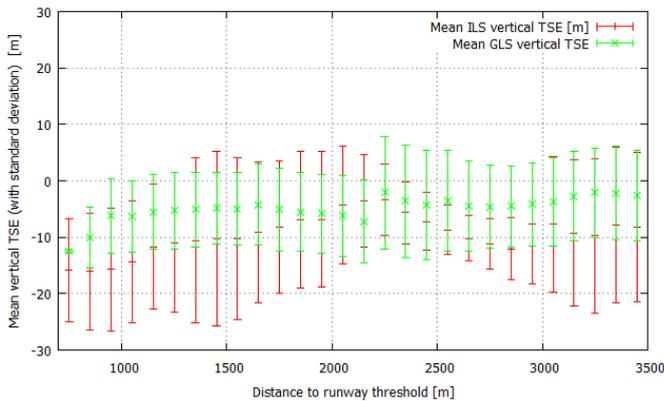
Figure 15: Comparison of mean vertical TSE during ILS (red) and GLS (green) approaches
