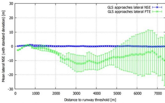
Figure 9: Mean lateral FTE and NSE during GLS approaches
