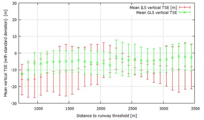
Figure 15: Comparison of mean vertical TSE during ILS (red) and GLS (green) approaches
