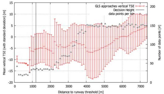
Figure 8: Mean vertical TSE during GLS approaches
