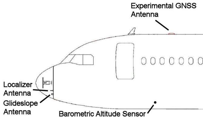
Figure 3: Approximate antenna and sensor positions
