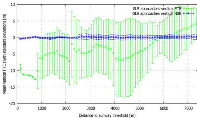
Figure 10: Mean vertical FTE and NSE during GLS approaches
