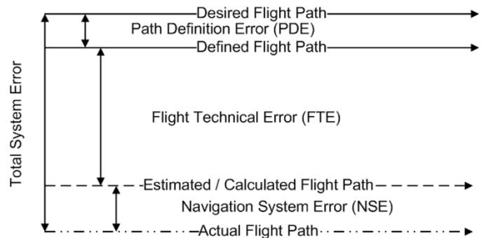
Figure 1: Flight Path Error Types
