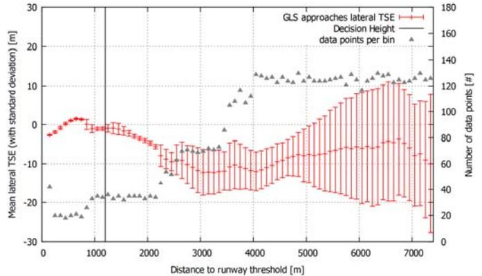
Figure 7: Mean lateral TSE during GLS approaches
