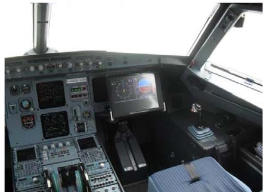
Figure 2: ATRA experimental cockpit display
