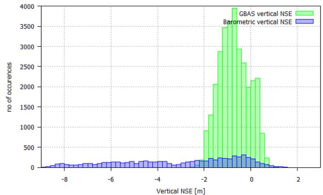
Figure 13: NSE distribution during the approaches of a single flight (GBAS, green and barometric altitude, blue)
