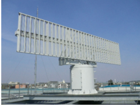
Figure 1. ENRI's SSR mode S Experimental Ground Station.
