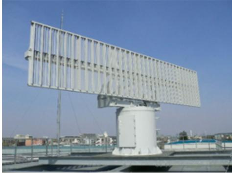
Figure 1. ENRI's SSR mode S Experimental Ground Station.
