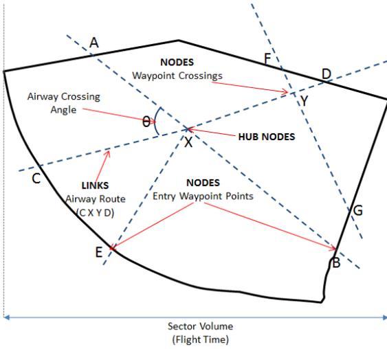
Figure 1: Airspace network modelled as a graph (network), comprising of waypoint as vertices or nodes linked by airways (links) connecting them.
