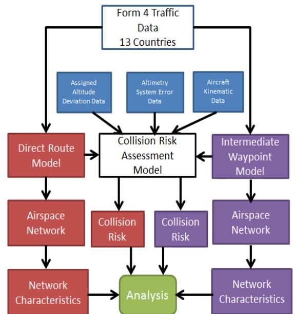
Figure 2: Proposed methodology for network characteristics analysis of direct route model and intermediate waypoint model for technical vertical risk.
