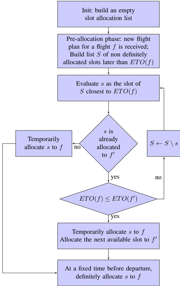
Fig. 3: Mechanics of CASA over a regulated area
