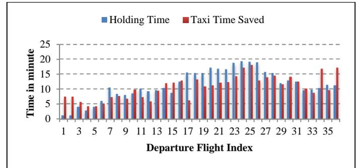
Figure 5 Holding time and excessive taxiing time reduced for departure flight
