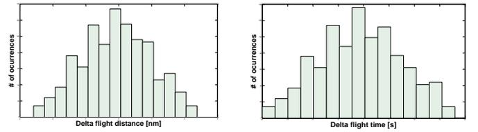
Figure 8. Distributions of  $\Delta d$  and  $\Delta t$  at the end of the trajectory
