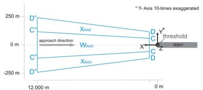
Figure 10. determined ANP- based OAS final approach surface – top view
