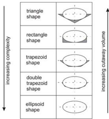
Figure 8. potential surface shapes
