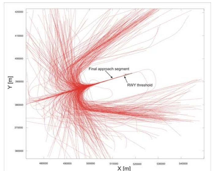
Figure 1. flight track snapshot – ILS approach
