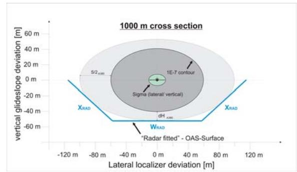
Figure 9. exemplary surface modelling for 1.000 m cross section
