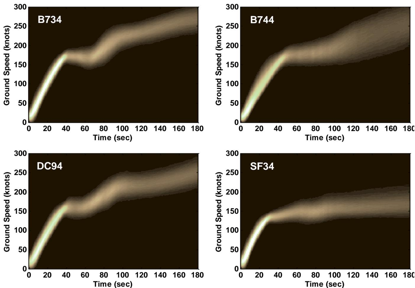
Figure 9. Two-dimensional pdf of PCA decomposition model for various aircraft types.
