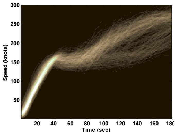
Figure 8. Two-dimensional pdf of DC10 departure ground speed trajectory from track data.
