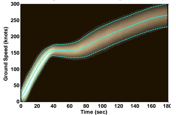
Figure 7. Two-dimensional pdf of A319 PCA decomposition trajectory model.
