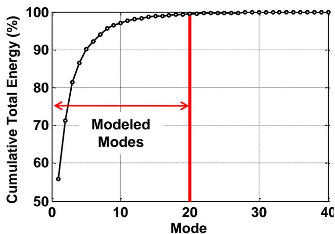
Figure 5. Cumulative total energy in the A319 PCA decomposition.
