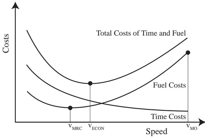
Figure 2. Impact of speed on operating costs
