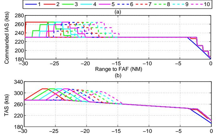
Fig. 11: Commanded IAS (a) and TAS (b) for a six-second initial spacing error between the first and second aircraft. The control law is updated every 15 seconds (compared to the 0.1-second update rate in previous results).
