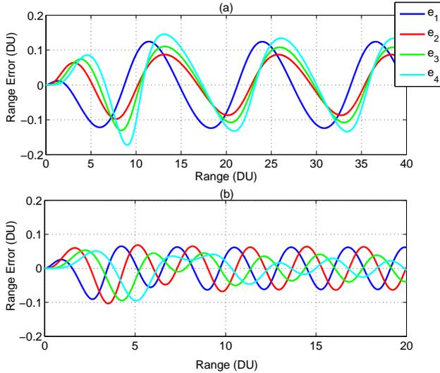
Fig. 2: Spacing errors between aircraft pairs when the first aircraft in the string is subject to a sinusoidal disturbance: (a)  $\omega = 0.5$  rad/sec, and (b)  $\omega = 2$  rad/sec.
