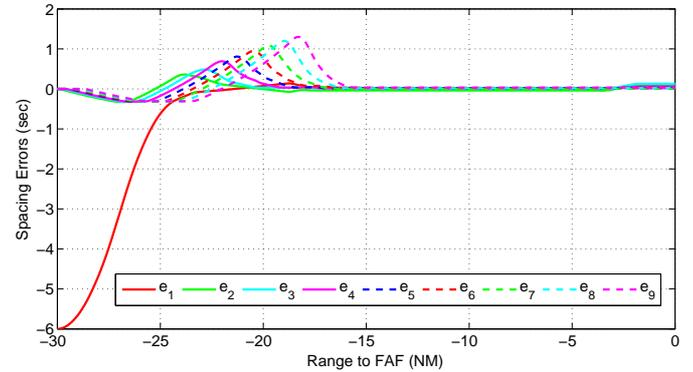
Fig. 8: Spacing errors as a function of range to FAF for a six-second initial spacing error between the first and second aircraft. Speed limitations are assumed.
