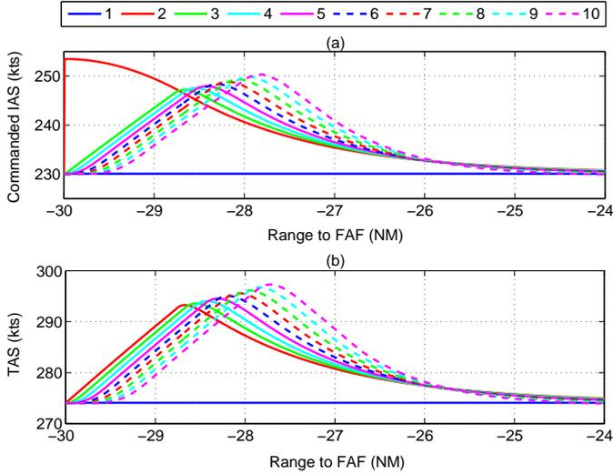
Fig. 6: Commanded IAS (a) and TAS (b) for a two-second initial spacing error between the first and second aircraft. Speed limitations are not imposed in the algorithm.
