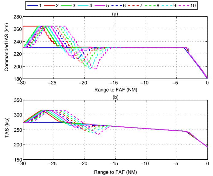
Fig. 7: Commanded IAS (a) and TAS (b) for a six-second initial spacing error between the first and second aircraft. Speed changes are limited to changes greater than  $\pm 2$  kts, speed commands are limited to  $\pm 15\%$  of the reference speed and are rounded to the nearest integer.
