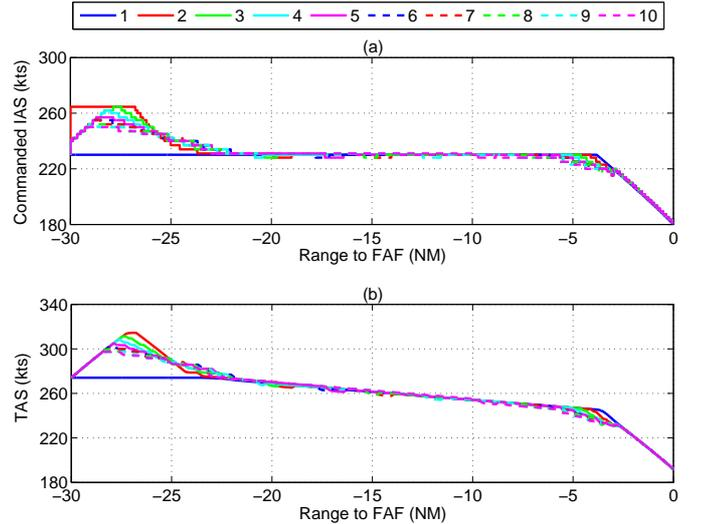
Fig. 12: Commanded IAS (a) and TAS (b) for a six-second initial spacing error between the first and second aircraft. The control law uses a spacing-anticipation parameter  $\tau_{sa} = 10$  seconds.
