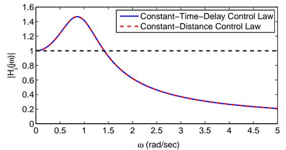
Fig. 1: Frequency response of the spacing-error transfer functions: time-history (blue solid line) and constant-distance (red dashed line) control laws.
