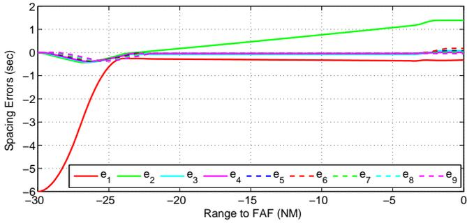
Fig. 10: Spacing errors as a function of range to FAF for a six-second initial spacing error between the first and second aircraft. Speed limitations and deadbands on the estimated spacing error are assumed.
