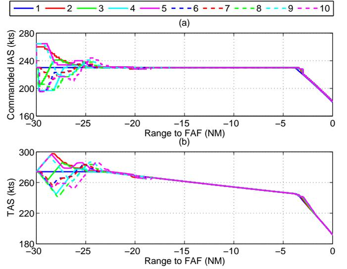
Fig. 4: Commanded IAS (a) and TAS (b) for Gaussian-distributed initial spacing errors. The speed-control algorithm includes speed limitations, assumes a realistic ADS-B update rate, and assumes frequent control-law updates.
