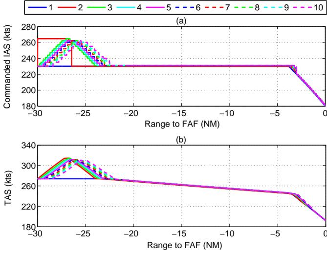
Fig. 9: Commanded IAS (a) and TAS (b) for a six-second initial spacing error between the first and second aircraft. The control law includes speed limitations and deadbands on the estimated spacing error.
