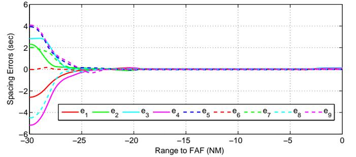
Fig. 5: Spacing errors as a function of range to FAF for Gaussian-distributed initial spacing errors.
