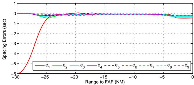
Fig. 13: Spacing errors as a function of range to FAF for a six-second initial spacing error between the first and second aircraft. The control law uses a spacing-anticipation parameter  $\tau_{sa} = 10$  seconds.
