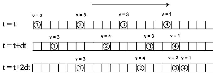
Figure 1. The patten diagram of NS model.
