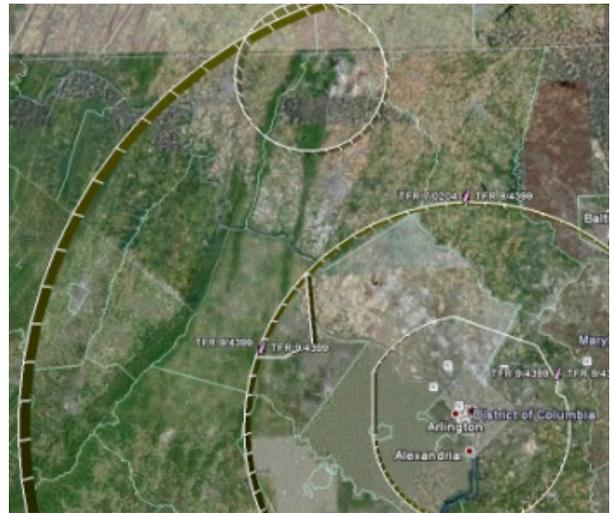
Figure 3. A more complex restricted airspace over the Washington, D.C. area is constructed using a combination of inner and outer cylinders, arcs, planes and cutouts.
