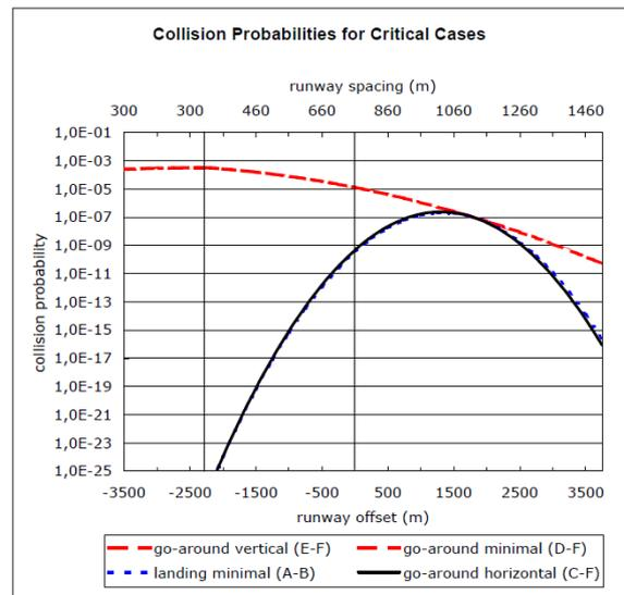
Figure 5. Collision probabilities for critical cases
