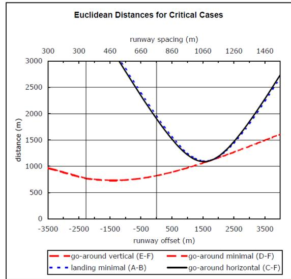
Figure 4. Minimal distances for critical cases in dependence of runway staggering
