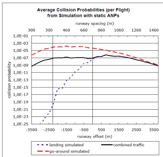
Figure 7. Average simulated collision probabilities for static ANP values
