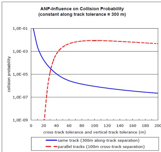
Figure 2. Influence of track keeping capability on collision probability
