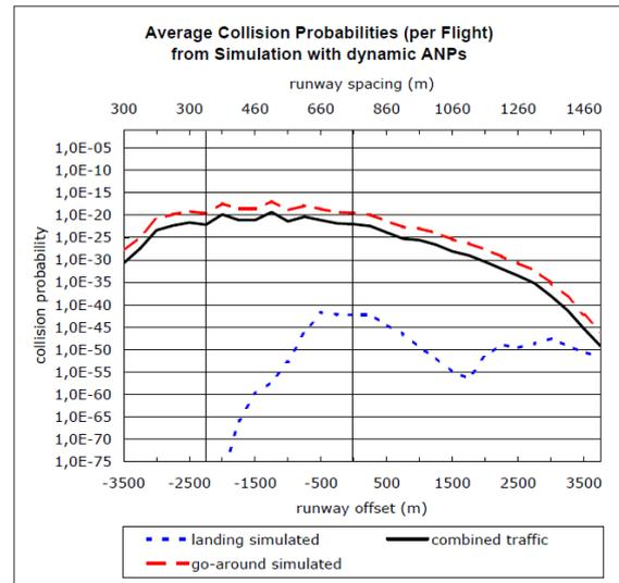
Figure 8. Average simulated collision probabilities for dynamic ANP values
