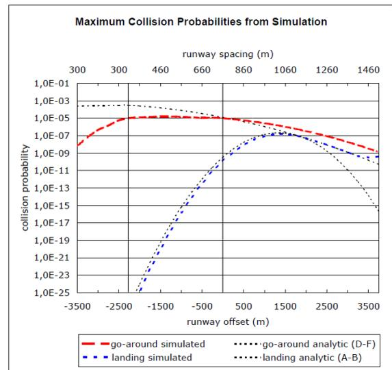
Figure 6. Maximum collision probabilities from simulation run
