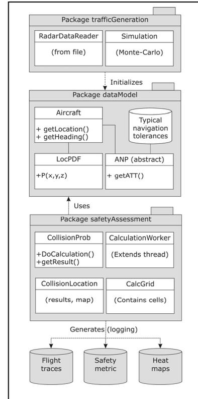
Figure 1. Safety Assessment Tool package structure (overview)
